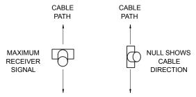
Trace the path by walking away from the Transmitter at a moderate pace. Move the Receiver to the left and right while walking, following the PEAK indications.
