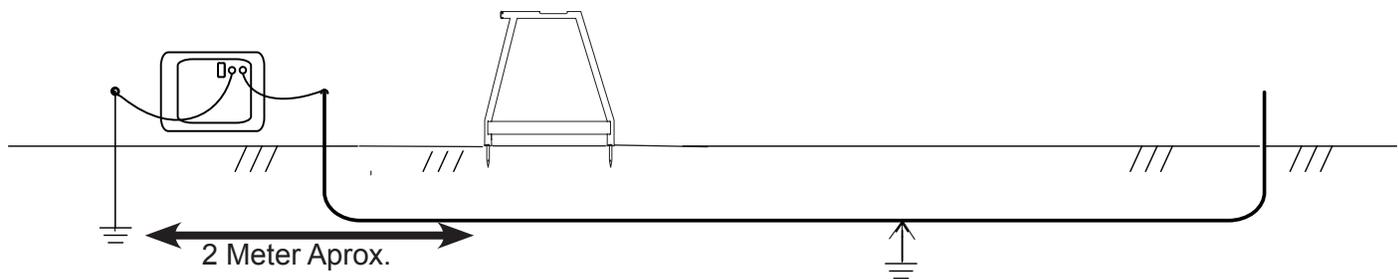
12) Signal strength will fall as leaving the ground spike until passing the half-way point between ground spike and fault. Signal will start to rise from half-way point to fault. If the distance is great the signal strength may fall to non-detectable level and arrows may not stabilize through the center section.
