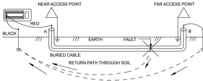
It is generally a good idea to locate the conductor path before attempting to fault locate. If, during the path locate, an unusual amount of signal loss occurs, a part of the signal has escaped to ground in the last several feet.
