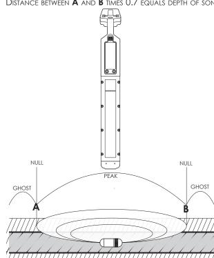
DISTANCE BETWEEN **A** AND **B** TIMES 0.7 EQUALS DEPTH OF SONDE.
