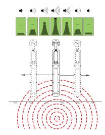
If you rotate the RECEIVER while over the cable, a sharp NULL will identify the cable's direction. It is aligned with the flat side of the RECEIVER.
