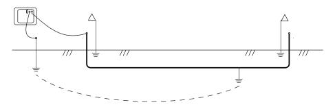
With transmitter off connect red lead to the faulted conductor and black lead to independent ground rod placed behind and in line with the conductor path.
