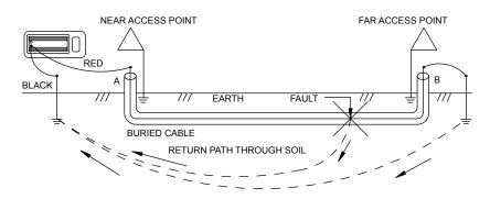
Set the Transmitter to fault mode by pressing and holding the frequency button for 10 seconds. When released the DFF symbol on the LCD will be displayed.
