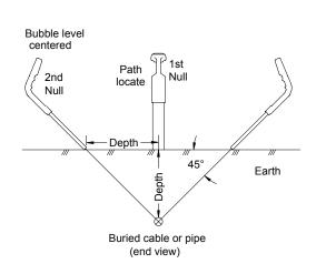
The only way to be sure of the depth of a utility is to exposes the utility. At any given time, the depth readout may be inaccurate.
