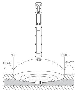
Start by following the suspected path of the pipe. Stop locating when the PEAK reading is found. Then rotate the Receiver as shown in the figure below. When pivoting the Receiver, do not change the vertical position. The Receiver will indicate a PEAK when the Receiver antenna is in line with the Sonde.
