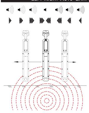
In this mode the unit will display directional arrows to the conductor. The audio indicator will provide a solid tone on one side of the conductor and a pulsed tone on the opposite side of the conductor. When the unit is centered in the electromagnetic field the tone will null and the depth will briefly display at the top of the LCD. This mode is gain independent.
